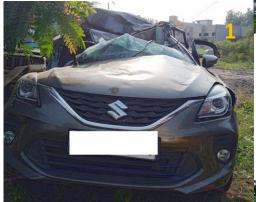
Collision damage mainly on the right side of vehicle. Other damage related to extrication and towing.
