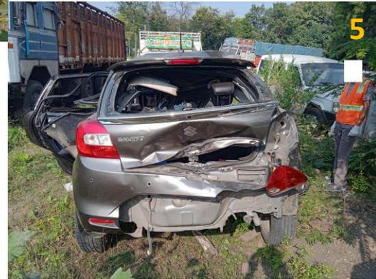
**Collision damage mainly on the right side of vehicle.
