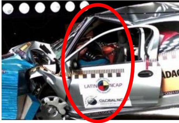
No airbag and poor body shell integrity gives zero stars. But just adding an airbag makes no difference...
