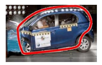
No airbag and poor body shell integrity gives zero stars. But just adding an airbag makes no difference...
