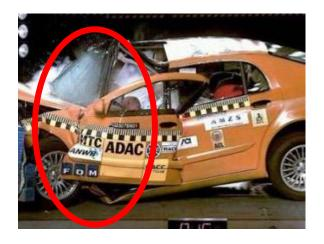
The combination of good body shell integrity and an airbag results in a survivable crash.
