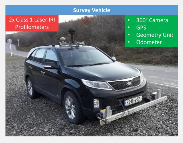
Road Condition Data collection by Laser Crack Measurement System
