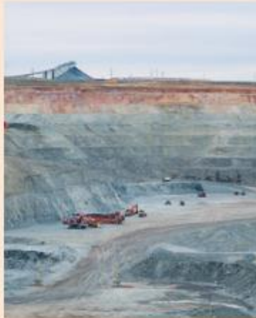
Pre-split drilling and blasting at Aktogay to preserve pit wall stability
