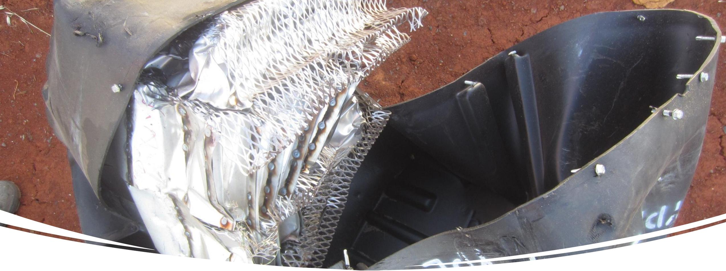
Inside an impact attenuator cartridge
