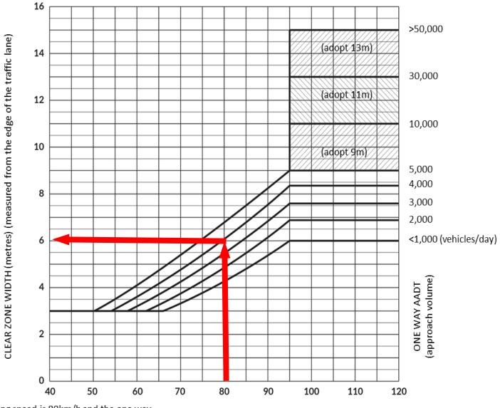
EXAMPLE 1 If the operating speed is 80km/h and the one way AADT is 4,000 vehicles/day, the clear zone width is 6m
