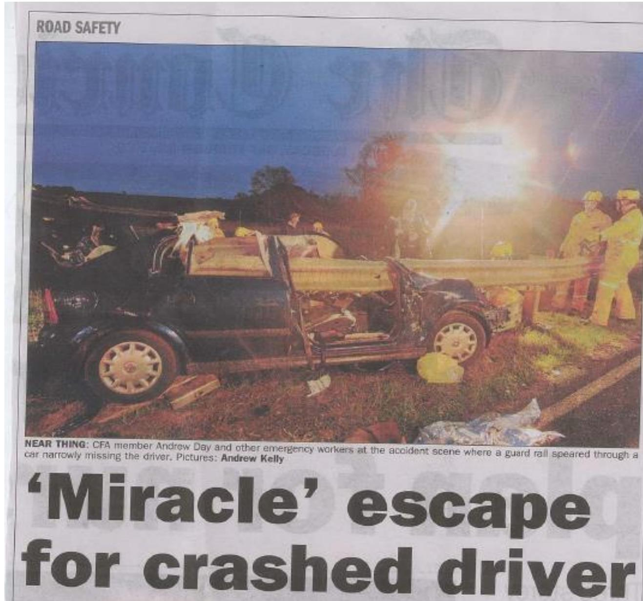
End treatments are necessary to avoid penetration into the vehicle
