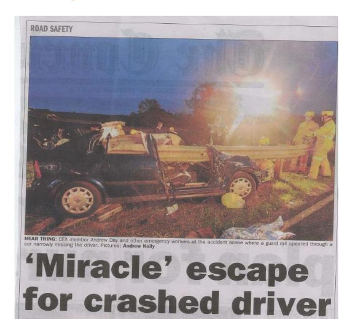
End treatments are necessary to avoid penetration into the vehicle
