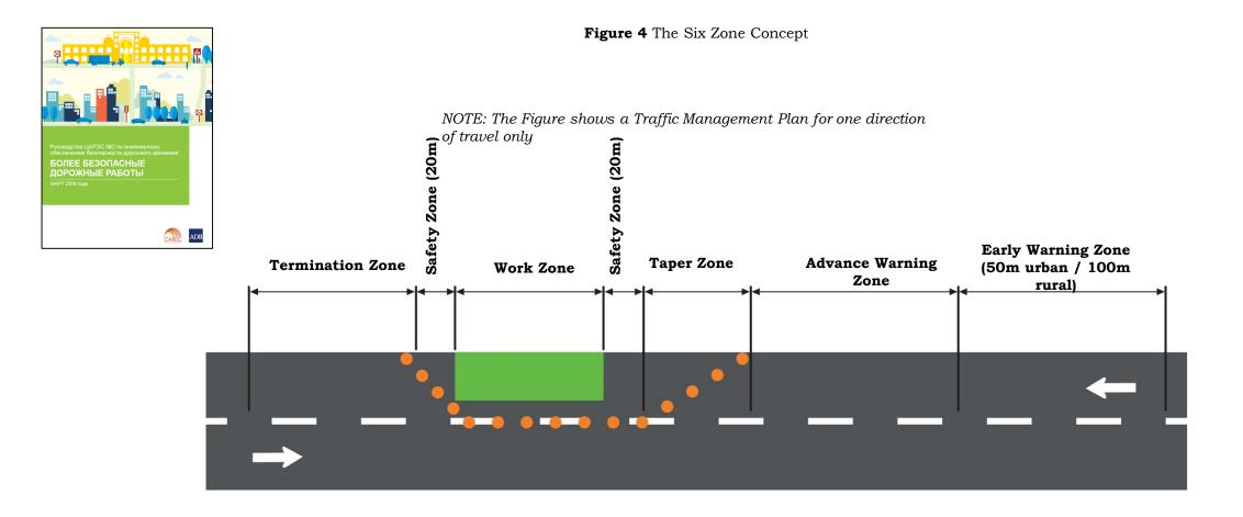
The CAREC Safer Road Works manual encourages the use of the six zone concept
